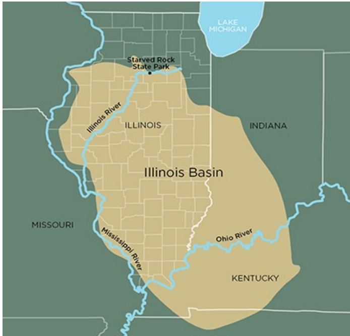
The Illinois Basin region which covers most of Illinois, southwestern Indiana, and western Kentucky with a storage capacity ranging between 12 billion to 172 billion metric tons of CO 2 . Source: Prairie Research Institute. November 2020.
