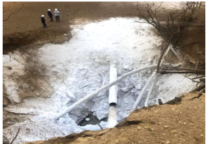
The CO2 pipeline rupture near Satartia created a crater 40 feet deep, hurled debris hundreds of feet into the air, and covered the area with ice. Photo courtesy of the Yazoo County Emergency Management Agency.
